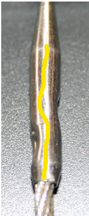
Fig 3 shows top view of both dimples forcing the cable into a S curve inside the pin
