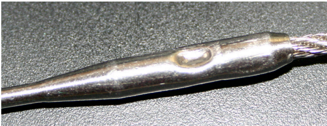
Fig 2 shows adjacent side of pin with offset dimple
